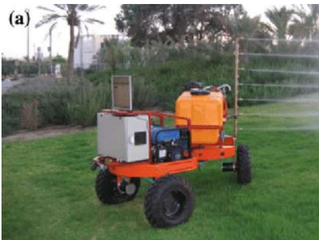
Berenstein, R., Shahar, O.B., Shapiro, A. et al. Grape clusters and foliage detection algorithms for autonomous selective vineyard sprayer. Intel Serv Robotics 3, 233–243 (2010). https://doi.org/10.1007/s11370-010-0078-z
